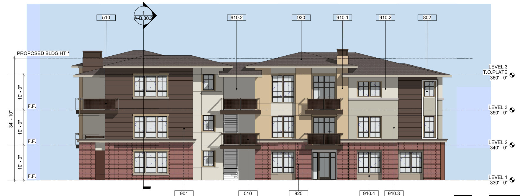
BUILDING B EAST ELEVATION 3/16" = 1'-0" 3
