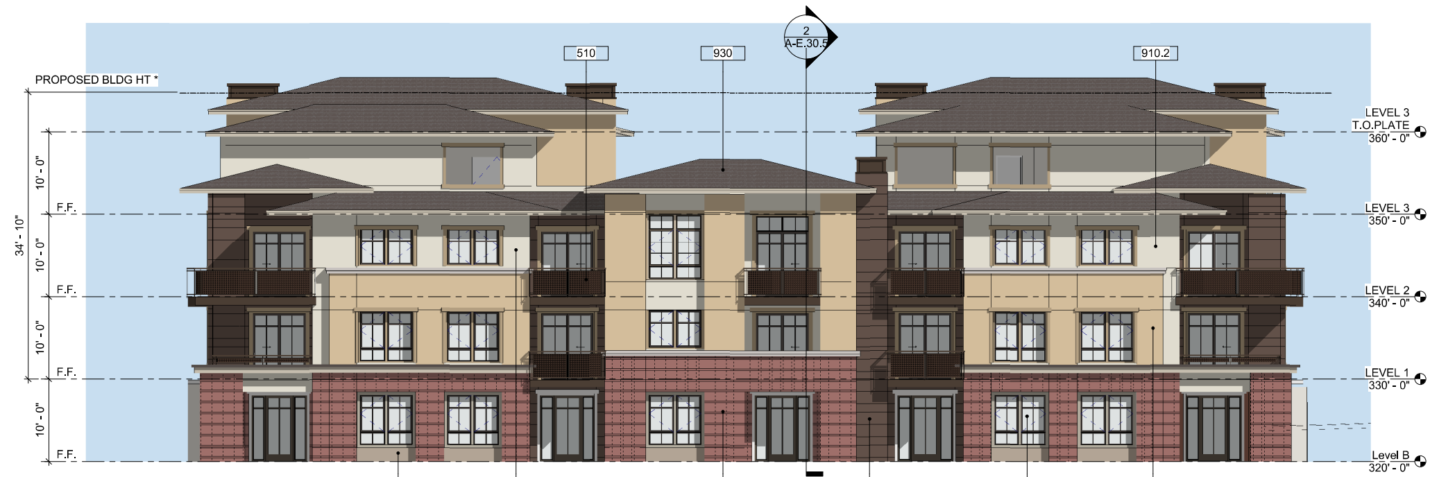
BUILDING E SOUTH ELEVATION 3/16" = 1'-0" 1
