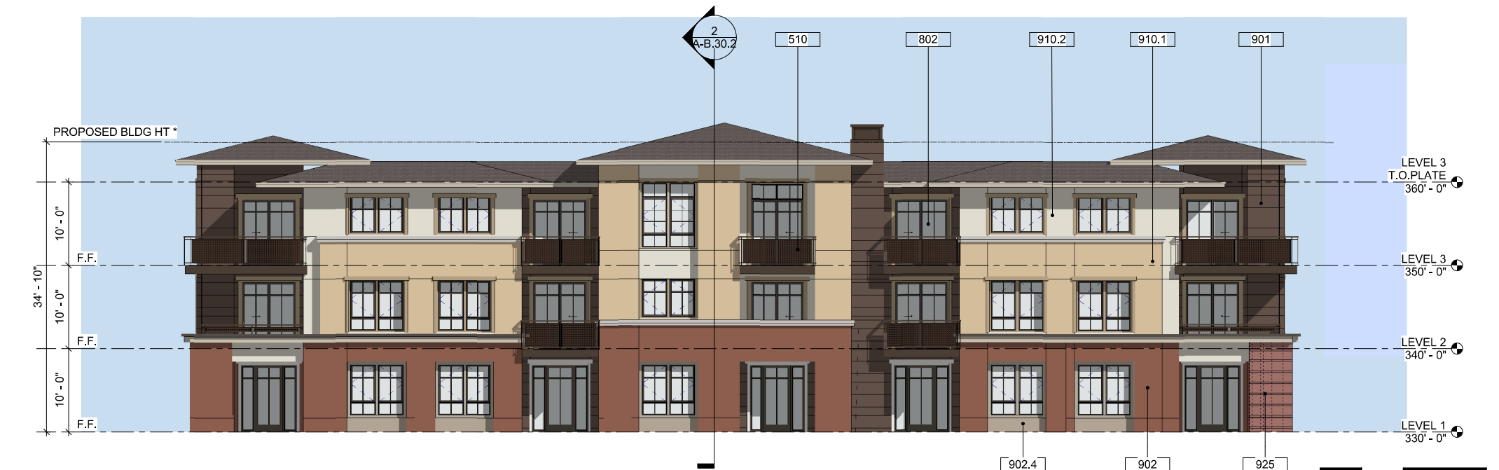
BUILDING B NORTH ELEVATION 3/16" = 1'-0" 1
