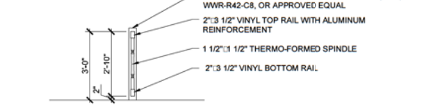
11 VINYL RAILING SECTION 3/8" = 1'-0"
