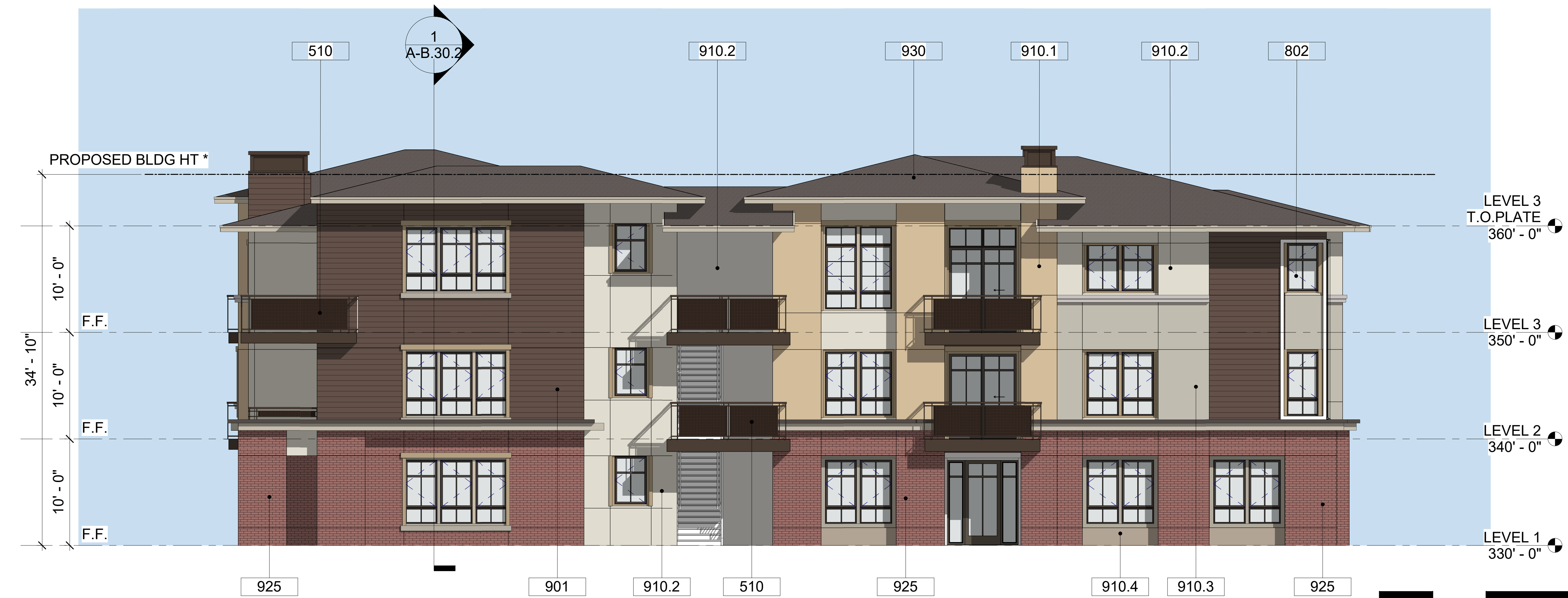
BUILDING B EAST ELEVATION 3/16" = 1'-0" 3
