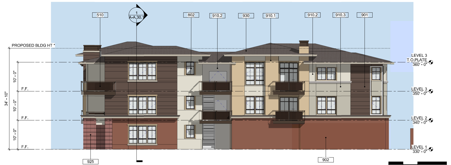
BUILDING A WEST ELEVATION 3/16" = 1'-0" 3
