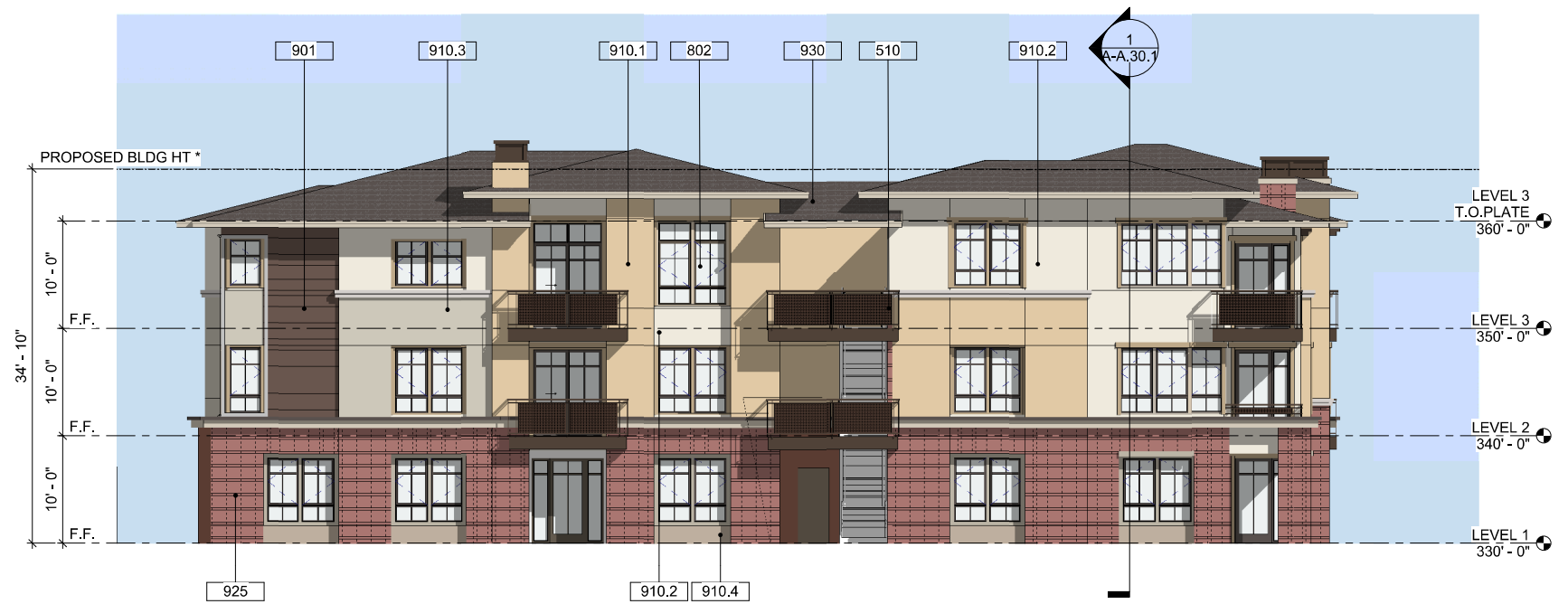
BUILDING A EAST ELEVATION 3/16" = 1'-0" 4
