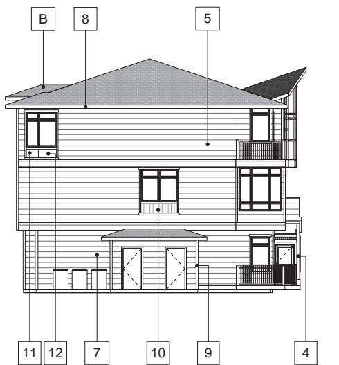
4 West Elevation, Materials 1/8" = 1'-0"
