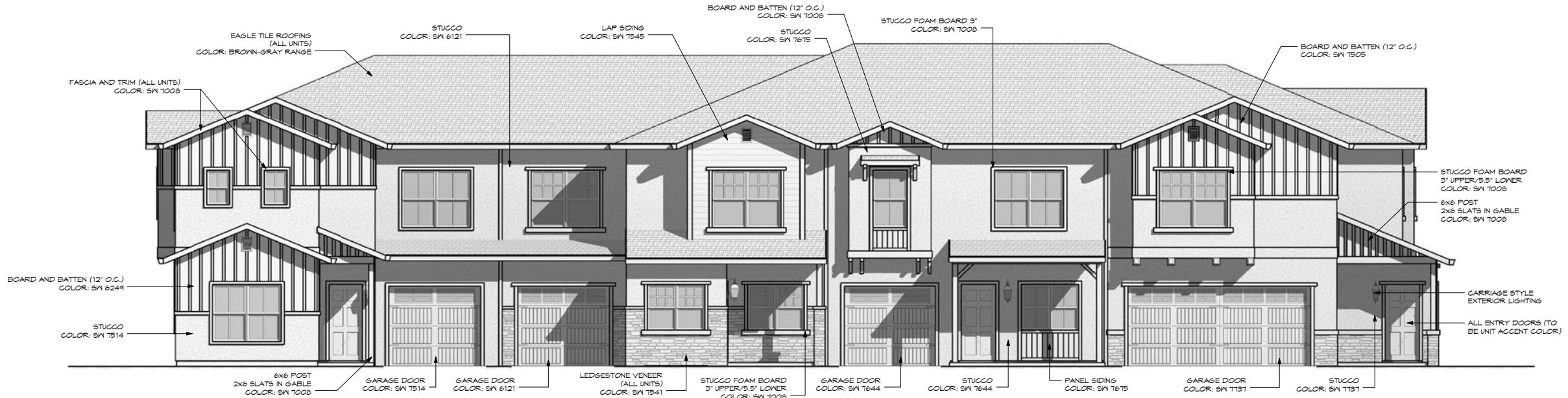
1 EXTERIOR ELEVATION - FRONT (4 PACK UNITS) SCALE: 1/4" = 1'-0"
