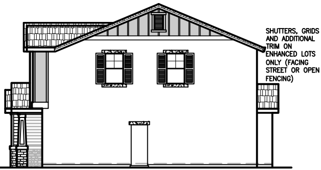
ENHANCED RIGHT ELEVATION 'B' SCALE: 1/16"=1'-0"
