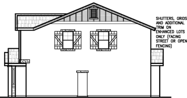
ENHANCED RIGHT ELEVATION 'B' SCALE: 1/16"=1'-0"
