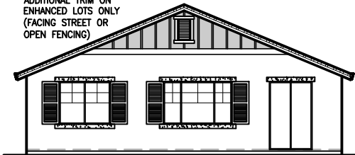
ENHANCED REAR ELEVATION 'B' SCALE: 1/16"=1'-0"
