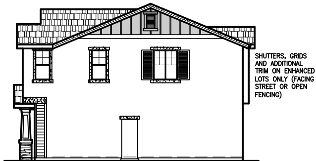
ENHANCED RIGHT ELEVATION 'B' SCALE: 1/16"=1'-0"
