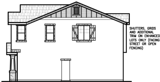
ENHANCED RIGHT ELEVATION 'B' SCALE: 1/16"=1'-0"
