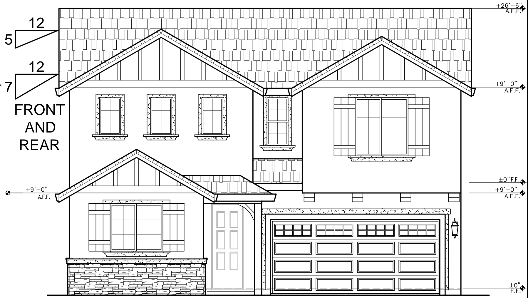
FRONT ELEVATION 'C' SCALE: 3/16"=1'-0"
