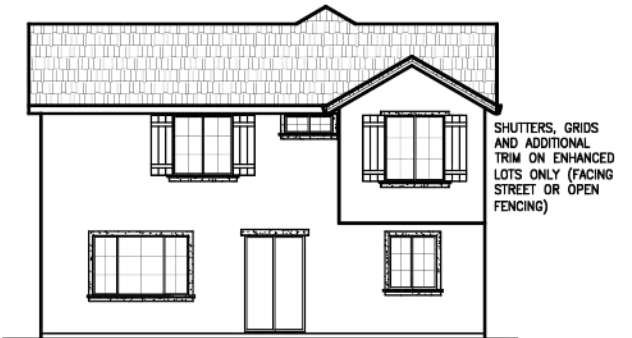
ENHANCED REAR ELEVATION 'C' SCALE: 1/16"=1'-0"
