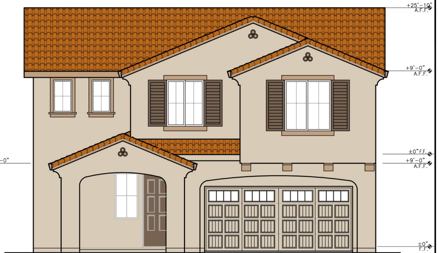
FRONT ELEVATION 'A' SCALE: 3/16"=1'-0"
