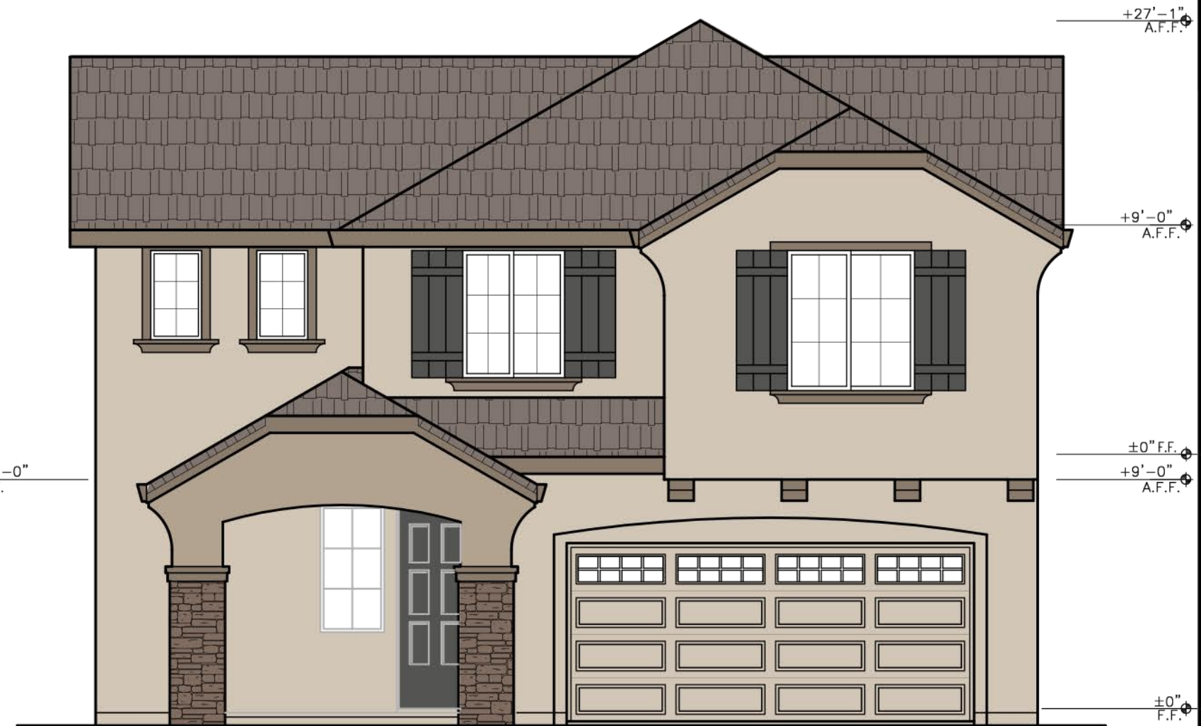
FRONT ELEVATION 'C' SCALE: 3/16"=1'-0"
