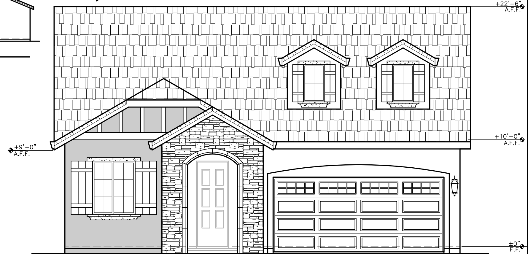
FRONT ELEVATION 'C' SCALE: 3/16"=1'-0"
