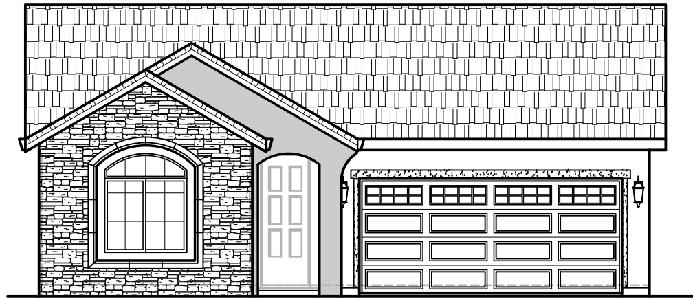
FRONT ELEVATION 'C' SCALE: 3/16"=1'-0"
