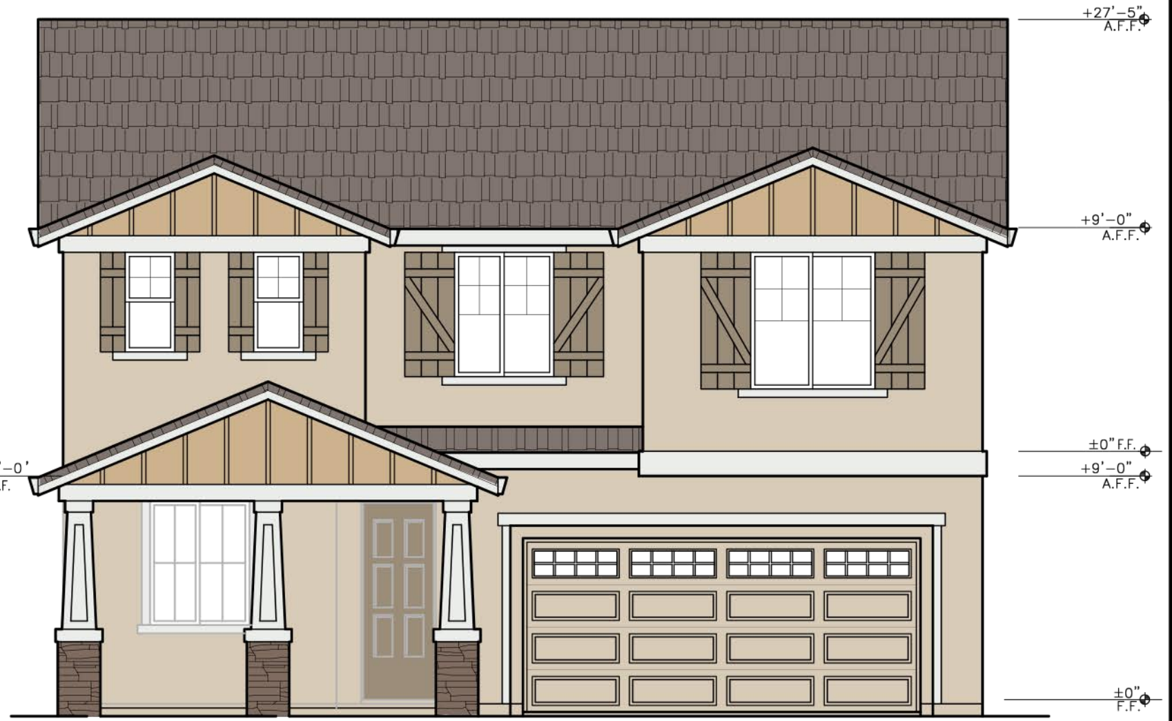
FRONT ELEVATION 'B' SCALE: 3/16"=1'-0"
