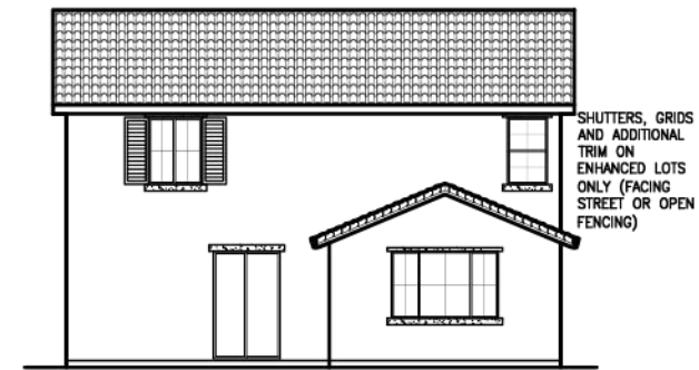
ENHANCED REAR ELEVATION 'A' SCALE: 1/16"=1'-0"
