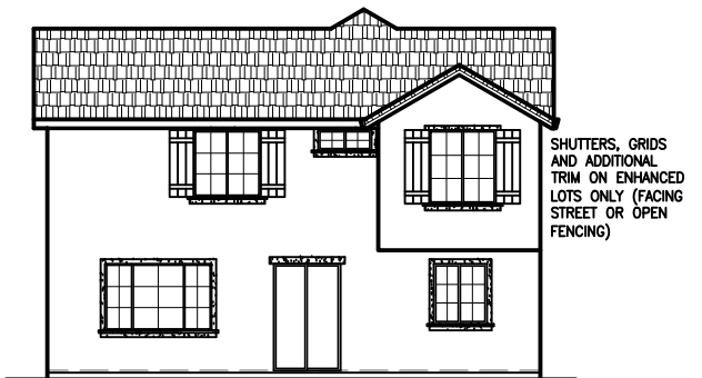
ENHANCED REAR ELEVATION 'C' SCALE: 1/16"=1'-0"
