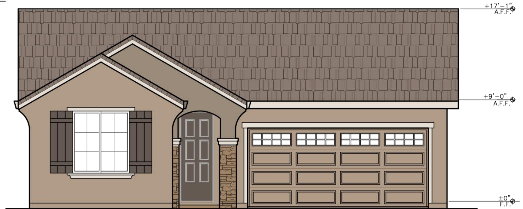
FRONT ELEVATION 'C' SCALE: 3/16"=1'-0"
