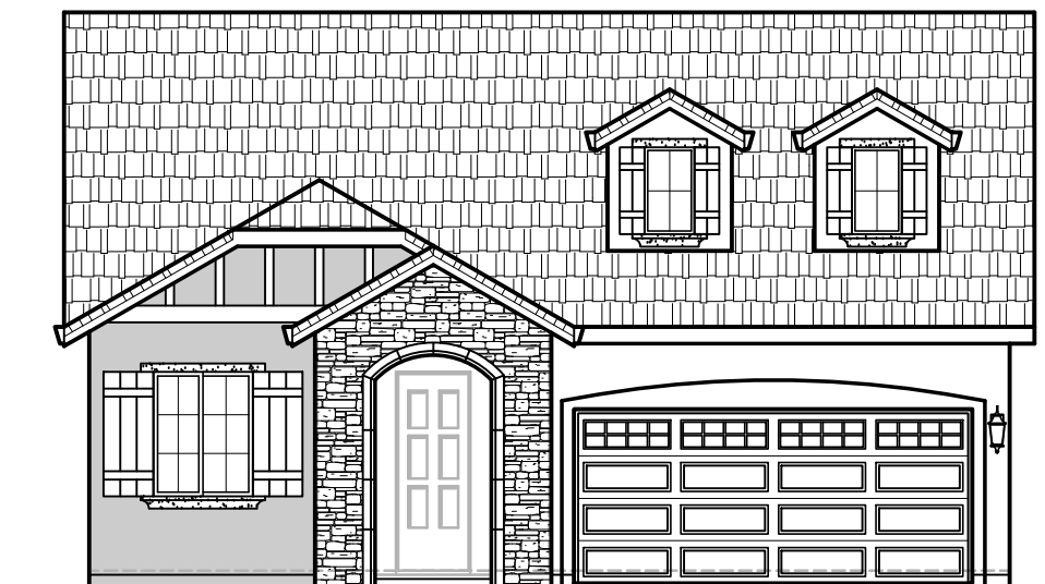
FRONT ELEVATION 'C' SCALE: 3/16"=1'-0"
