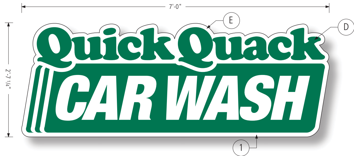
C Illuminated Pan Channel Shaped Cloud Sign Scale 3/4" = 1'-0" Sign Area: 18.1 sq.ft.
