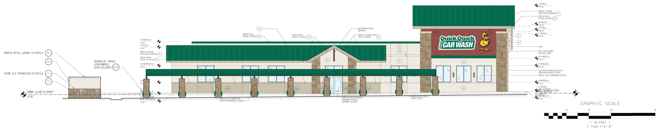
CANOPY ELEVATION (VIEW FROM STANFORD RANCH ROAD) SCALE: 1/8"=1'-0" 01
