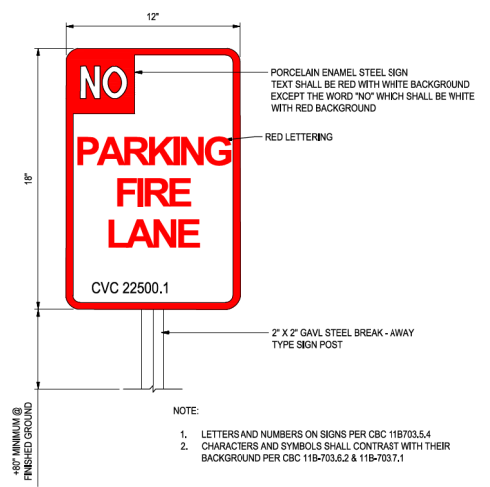
2 FIRE LANE SIGNAGE NO SCALE
