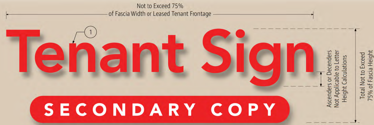
Single Line Letters with Shaped Cabinet Sign for Secondary Copy Not to Scale
